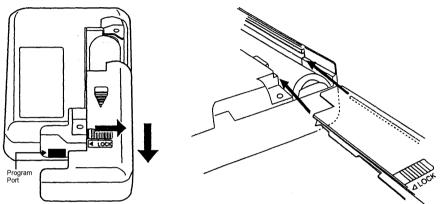
Note that when a new or working battery is installed, after about 2 seconds the alerter will turn on.
